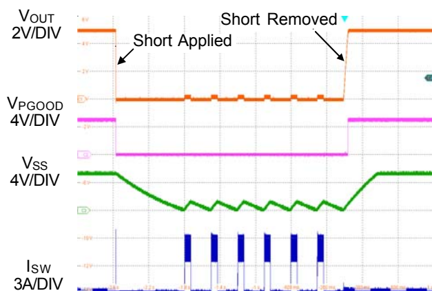
Figure 3. Short-Circuit Protection and Recovery
